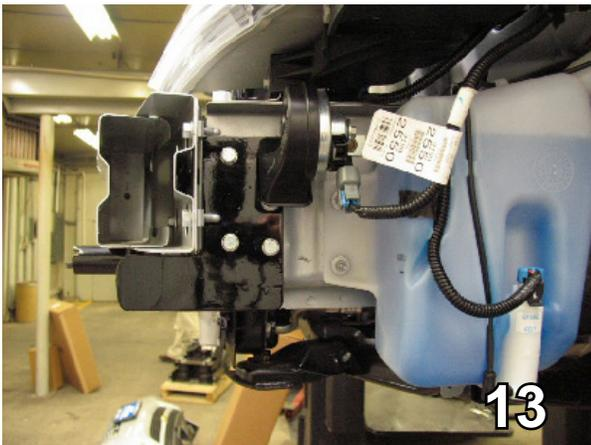
13. Reinstall horn bracket on the driver's side, using the existing equipment with the 10MM socket. **Be sure that all electrical connections are plugged in properly.**
