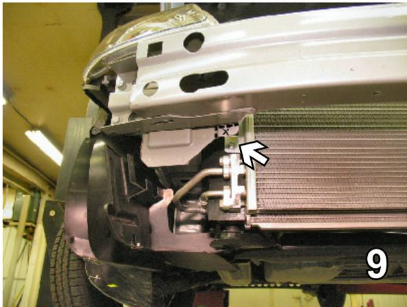
9. Mark a line from inner edge of bumper brace, along the bottom edge of metal bumper and down, flush with the inside edge of frame rail, both sides (view of passenger's side). Remove this area with the reciprocating saw, both sides.
