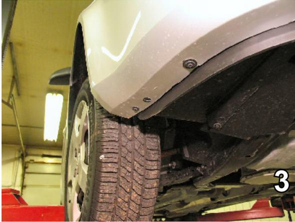
3. Remove the two metric bolts from lower edge of fascia, just forward of front tires with the 7MM socket, both sides.
