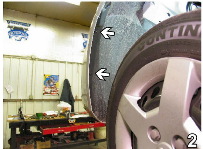
2. Just forward of front tire, on edge of wheel well, are three metric bolts to remove with the 7MM socket, both sides.
