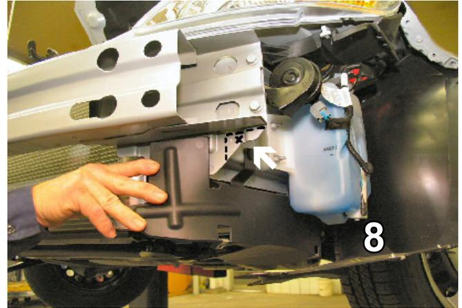
8. Mark a line from outer edge of bumper brace, along the bottom edge of metal bumper and down, flush with the outside edge of frame rail, both sides (view of driver's side). Remove this area with the reciprocating saw, both sides.
