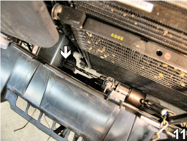
11. Using the baseplate as a template, drill two holes into the frame rail, between the radiator and the metal bumper, with the 13/32" drill bit. Do this to both sides of the vehicle.
