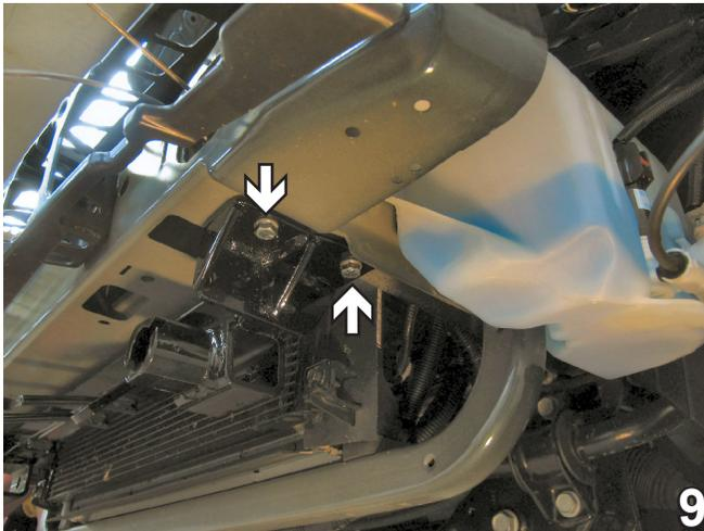
9. Align the baseplate with the two outside existing holes, where the tow hooks were connected to the frame rail, and clamp in place with the vise grips. Insert 3/8-16 x 1 1/4" hex bolts with 3/8" lock washers. Do this to both sides of the vehicle.
