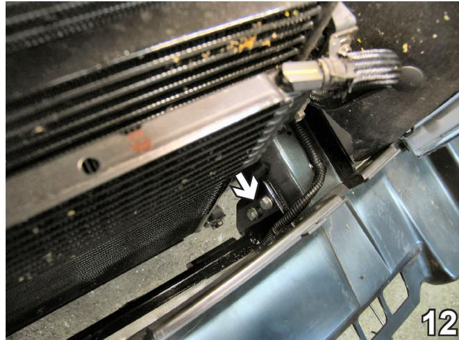
12. Install the 3/8-16 x 1 1/4" hex bolts with 3/8" lock washers into the drilled holes. Insert 3/8-16 nut plates into the frame rail opening and align with the bolts. Tighten all bolts. Do this to both sides of the vehicle.
