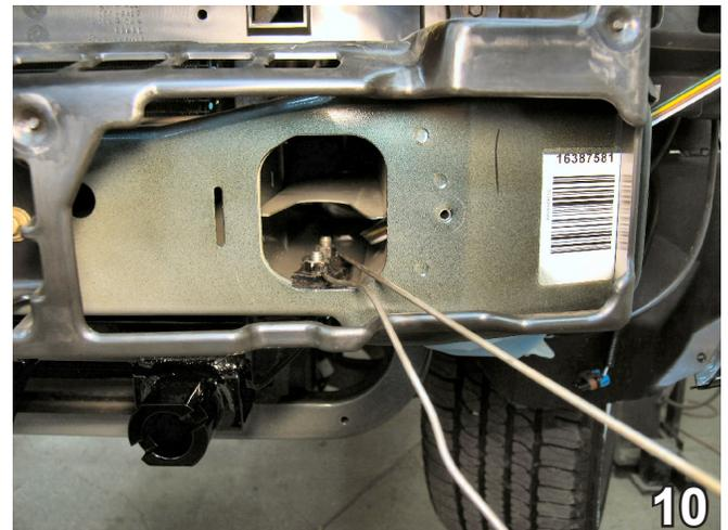
10. Install the backing plate onto the hex bolts followed by the 3/8-16 nut plates by inserting them through the frame cup opening and aligning with the bolts.
