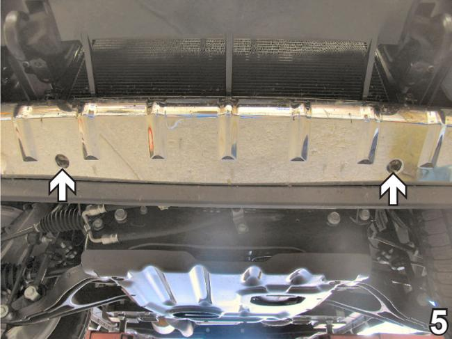
5. Using a 10MM socket, remove two metric bolts on the bottom side of the fascia. Set bolts aside to be reinstalled later.
