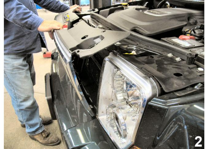
2. Pull up on the black plastic on the top of the fascia to release. Lift grille straight up to remove. Set grille aside to be reinstalled later.
