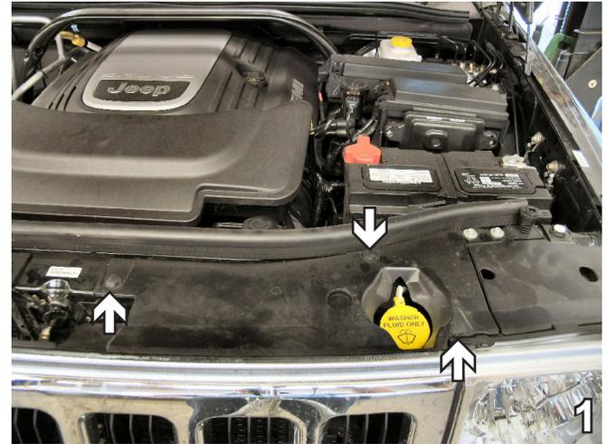
1. Remove six pushpins from the top of the fascia. Set pushpins aside to be reinstalled later. The driver's side is shown.
