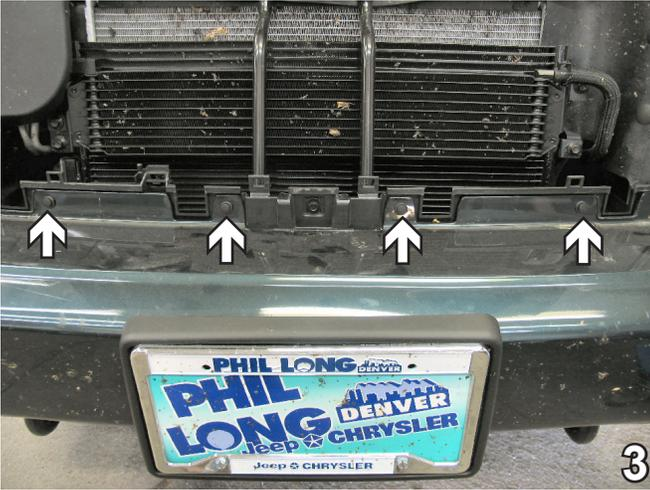
3. Remove four pushpins from the top of front fascia. Set pushpins aside to be reinstalled later.
