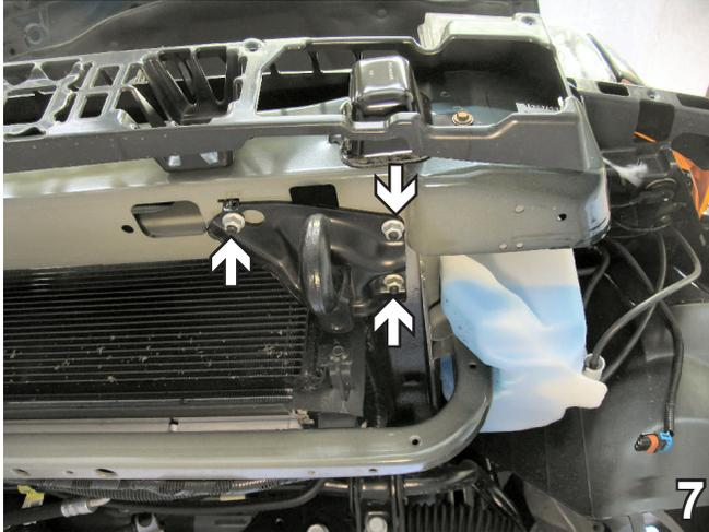
7. Using a 15MM socket, remove three metric nuts from the tow hook. Do this to both sides of the vehicle. The tow hooks will **NOT** be reinstalled, make sure that these are returned to the customer.
