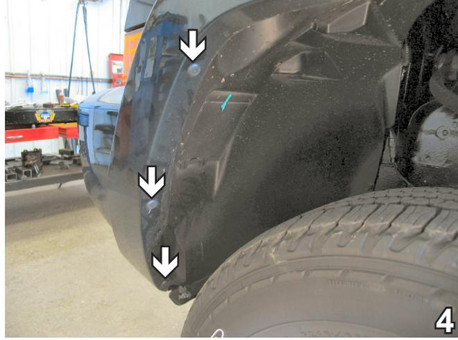
4. Just forward of the front tire, inside the wheel well, remove three rivets with the diagonal cutters. Discard rivets as new rivets are provided for reinstallation of the fascia.
