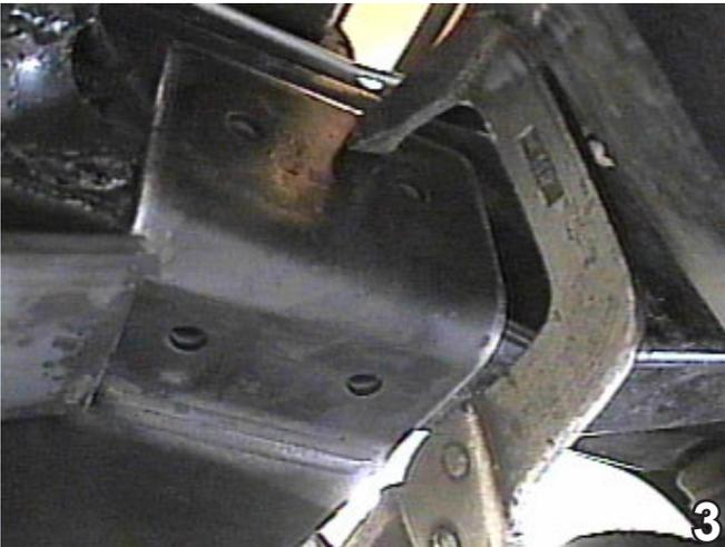
3. Clamp the baseplate on the passenger's side with the large vise grips. Using the baseplate as a template, drill four (4) holes with the 13/32" drill bit.
