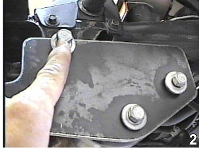
2. Hold the baseplate into place and insert the three (3) existing bolts on the driver's side through the baseplate, frame and gear box. Tighten the bolts.
