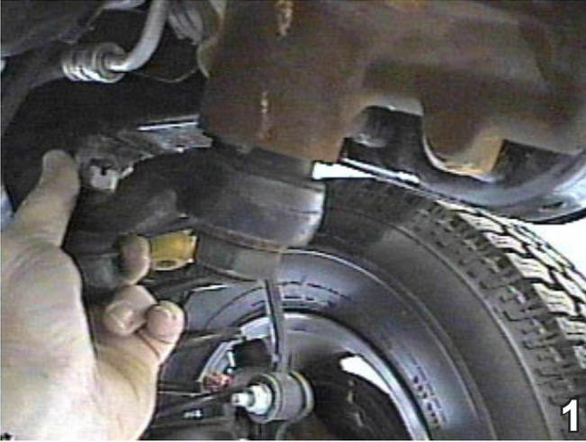
1. Remove three (3) metric bolts with the 16MM socket while having someone hold the gear box and the idler arm. Set metric bolts aside to be reinstalled later. Do this to both sides of the vehicle.
