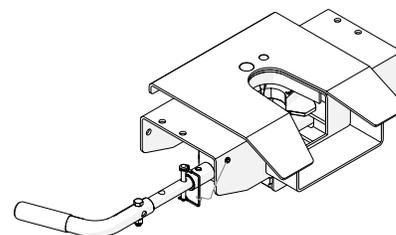
To uncouple, remove safety pin, pull handle straight out until the jaw locks open. If jaw will not stay open, install safety pin in second handle hole just outside of frame handle bushing.
