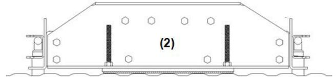
Once the hitch is installed and locked into place in the truck bed, adjust the height of the outrigger bar so that it is snug up against the top of the truck bed and tighten both nuts to lock into place.
