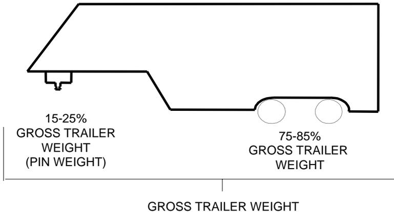
4. Trucks come in many different configurations. The Reese 30K fifth wheel is designed for medium duty truck applications such as Freightliner or Ford F-650. It is NOT intended for light duty pick-up trucks.
