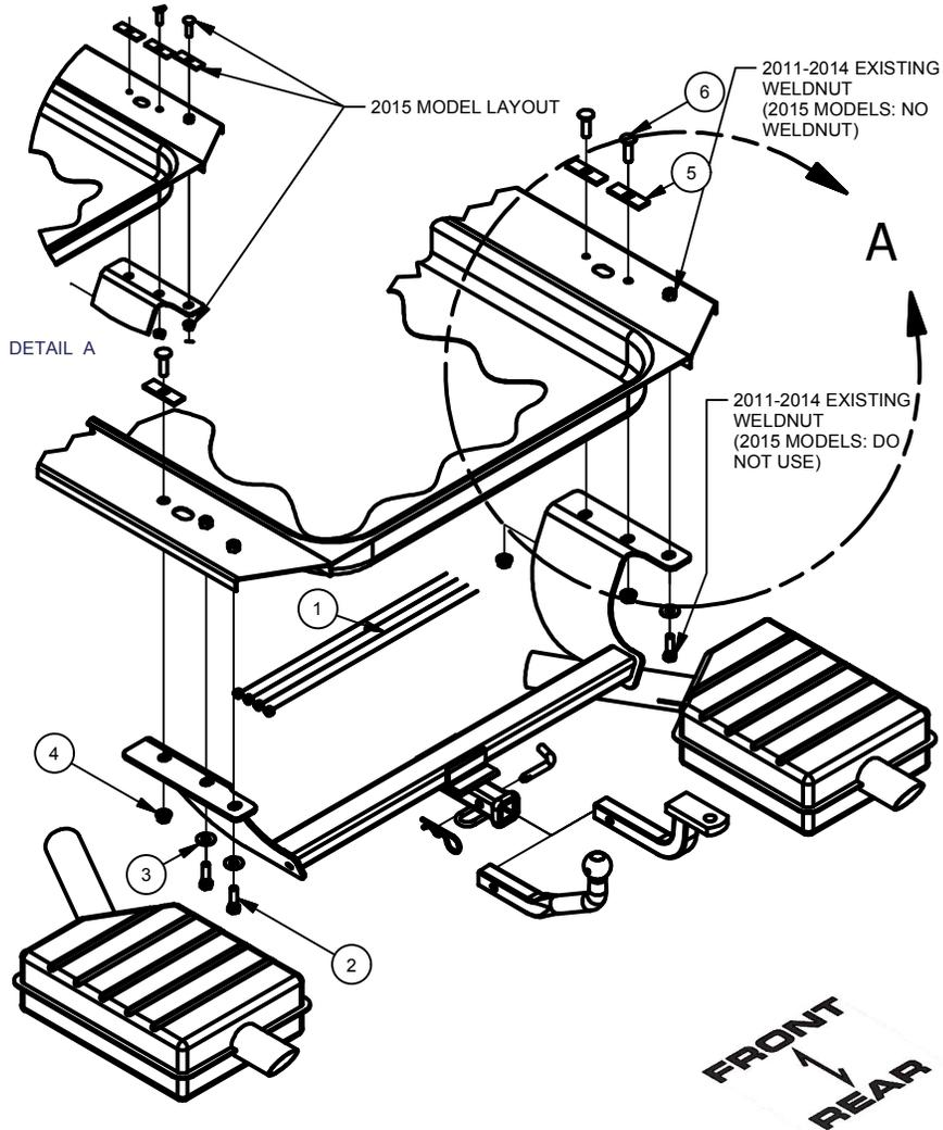
1. Locate and remove (2) exhaust isolators near muffler on driver and passenger side of vehicle. Save bolts for reinstallation.
